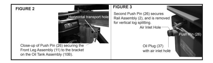
Rail Assembly must always be secured in the horizontal position for travel. Cover the air inlet hole on the Oil Plug (37) before transport. See FIGURE 3.
